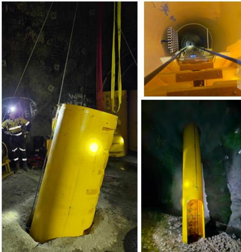
Figure 1 Secondary means of egress established using Safescape ladder system
